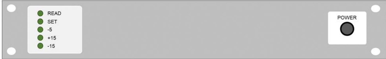
Fig. 1: Front view of the CR1000 box (top). Green circles represent various lights, while grey circles represent the circuit breakers.
