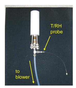
The new configuration is shown below. Water can collect in a long drain tube that needs to be inspected regularly and emptied and the T/RH probe enters the air stream from above, thereby lessening the chance that water drops will collect on the sensors.
