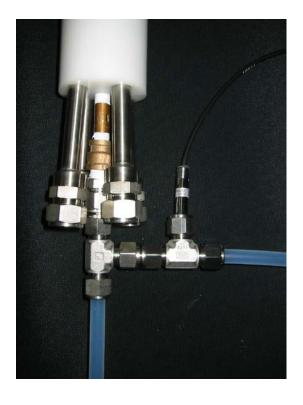
Close up view of the new splitter probe configuration is shown above.
