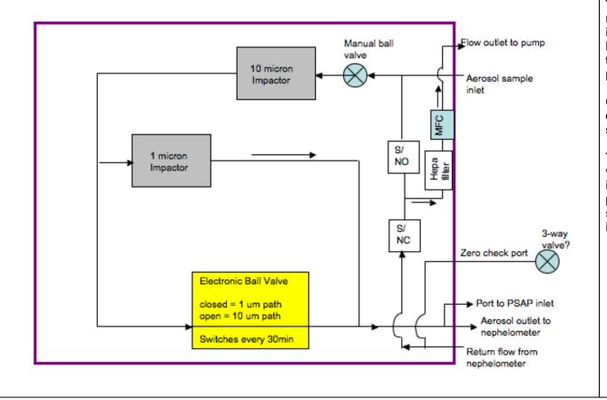
This schematic shows one way (the normal way) air can flow through the impactor box. If a span check is happening or the system is bypassed then different there are different flow paths.
