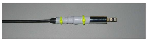
Sensor connection point wrapped for protection against elements. Silicon stretchy electrical tape was used.
