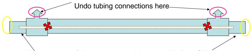
Unscrew these fittings to remove drier assembly from CN box, Once those are removed you should be able to see the tips of the nafion drier. Remove the o-rings and then pull the nafion drier tube out Do not undo the fittings marked with red crosses.
