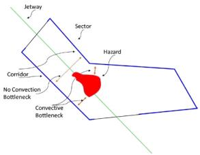
**Figure 2:** Illustration of the Mincut Bottleneck technique for a jetway,
