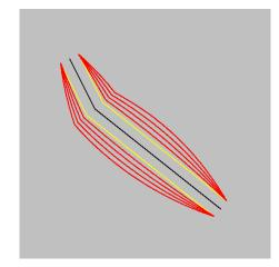
**Figure 3.** An example of "flexible" corridors with varying degrees of freedom (red lines) away from the route (black) with the original corridor (yellow).
