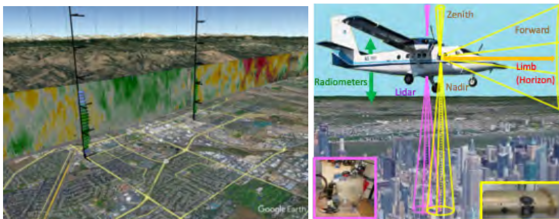
Figure 24: Example of airborne Doppler lidar vertical velocity data. (Left) and sensing volumes of remote measurements made from the NOAA Twin Otter during CUPiDS 2023 (Right).
