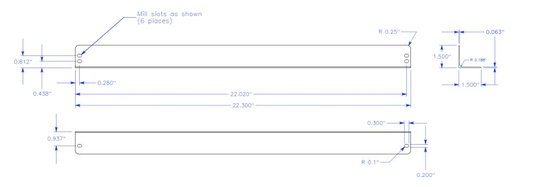
hole center—to—center distances measured at multiple points on 3 of 5 CSD racks (21.640" min. to 21.840" max.)
