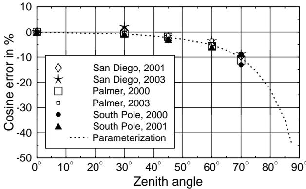
**Figure S2.** Cosine error ( $f_B(\theta) - 1$ ) of SUV-100 spectroradiometers with modified collector. The symbols represent measurements with the cosine test apparatus. The parameterization indicated by the dashed line was established with South Pole data from 2000 by comparing measured and modeled irradiance at 600 nm as explained in the text.
