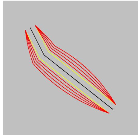
**Figure 3.** An example of “flexible” corridors with varying degrees of freedom (red lines) away from the route (black) with the original corridor (yellow).
