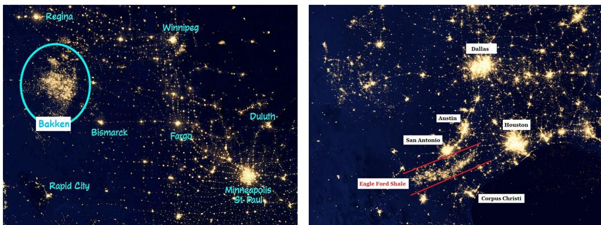
**Figure 7:** Gas flaring in the Bakken in North Dakota (left) and Eagle Ford shale in Texas (right) as observed from the Visible Infrared Imaging Radiometer Suite (VIIRS) satellite instrument (NOAA National Geophysical data Center)
