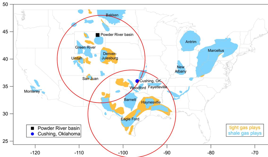
**Figure 6:** SONGNEX flight objectives. Tight sand and shale plays are shaded. The black square shows the location of surface coalmines in the Powder River Basin, Wyoming. The blue circle shows the location of a major intersection in crude oil pipelines near Cushing, Oklahoma. The open red circles show the range of the NOAA WP-3D for flights that take off and land from airfields in the Denver area in Colorado and a location to be determined in Texas.
