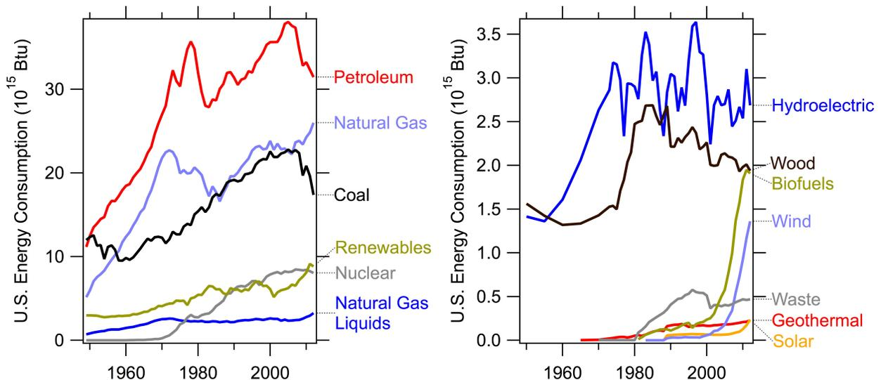
**Figure 1:** Energy consumption in the U.S.: all sources on the left and renewable energy sources on the right (data from the Energy Information Administration). Energy production is very similar, except for petroleum, of which a large fraction is imported
