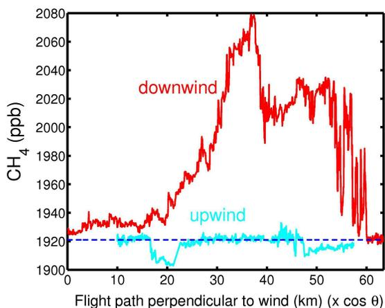
**Figure 3:** Airborne measurement of methane up- and downwind from oil and gas production fields in the Uintah basin in Utah [Karion *et al.*, 2013]. Methane fluxes were determined from the difference in integrated methane between the up- and downwind plumes, multiplied by the orthogonal wind speed and depth of the atmospheric boundary layer.
