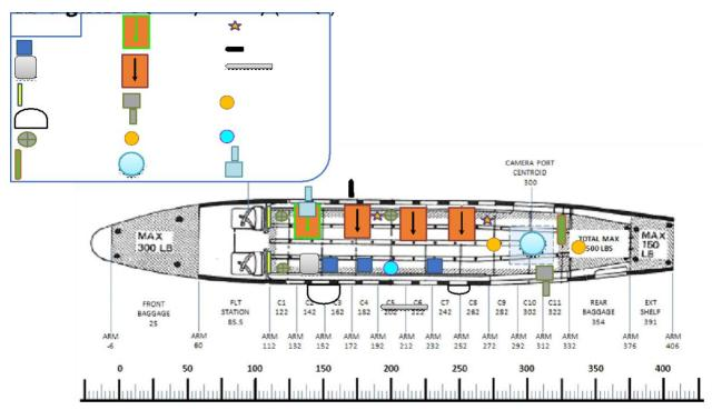
**Figure 2.** The proposed payload of the NOAA Twin Otter for the Baltimore Air Quality and Marcellus Methane Survey 2025.
