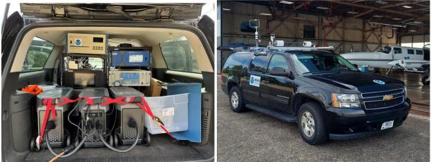
**Figure 4.** Pictures showing the instrumentation in NOAA's Air Resources Car mobile lab proposed for the Baltimore Air Quality and Marcellus Methane Survey 2025.
