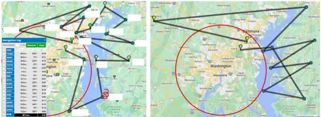
**Figure 7.** Examples of air pollution Lagrangian flight pattern over the Baltimore-Washington area planned for summer 2025.
